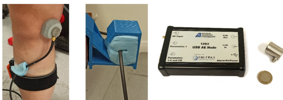
Figure 3. Testing setup: sensor fixation (left), cable fixation (center), USB AE Node monitoring system (right).
