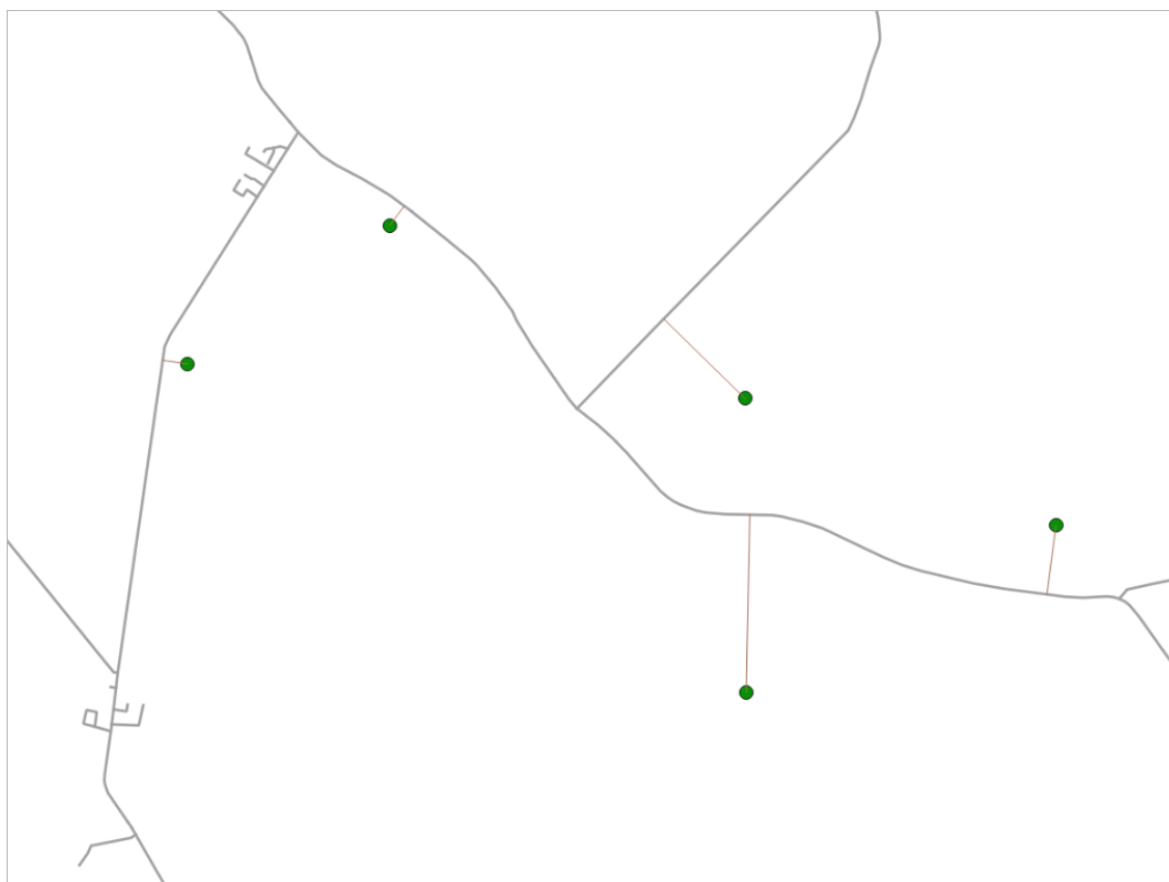
Figure D-16: Tangential lines from network nodes to road network layer.
