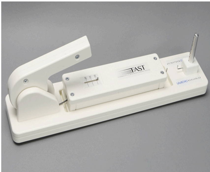
Figure 6.4 Fundamentals of Arthroscopic Surgery Training (FAST) knot tester. The suture loop is positioned on the 2 tines, and the handle allows for controlled application of 15 lb. of longitudinal load.
