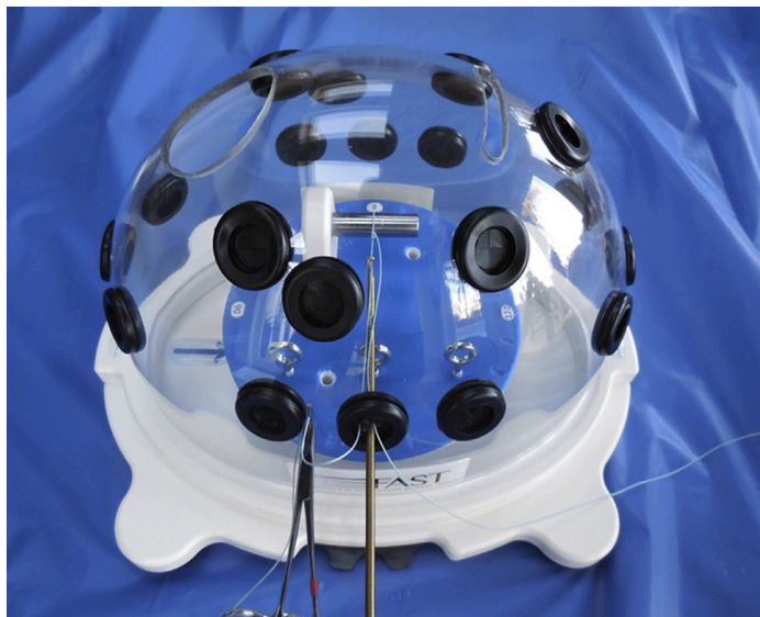
Figure 6.1 Fundamentals of Arthroscopic Surgery Training (FAST) base station with knot-tying mandrel and lucent dome for skills rehearsal under direct visualization.
