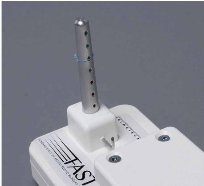
Figure 6.3 Conical loop sizer of Fundamentals of Arthroscopic Surgery Training (FAST) knot tester. The first mark indicates zero loop expansion, and each subsequent mark reflects 1 mm of additional loop expansion compared with the knot-tying mandrel.
