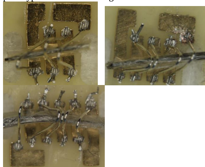
Figure 5. Fully assembled PCB thin film inductors (a)Design 1(N-3)(b)Design 2(N-4)(c)Design 3(N-5)
