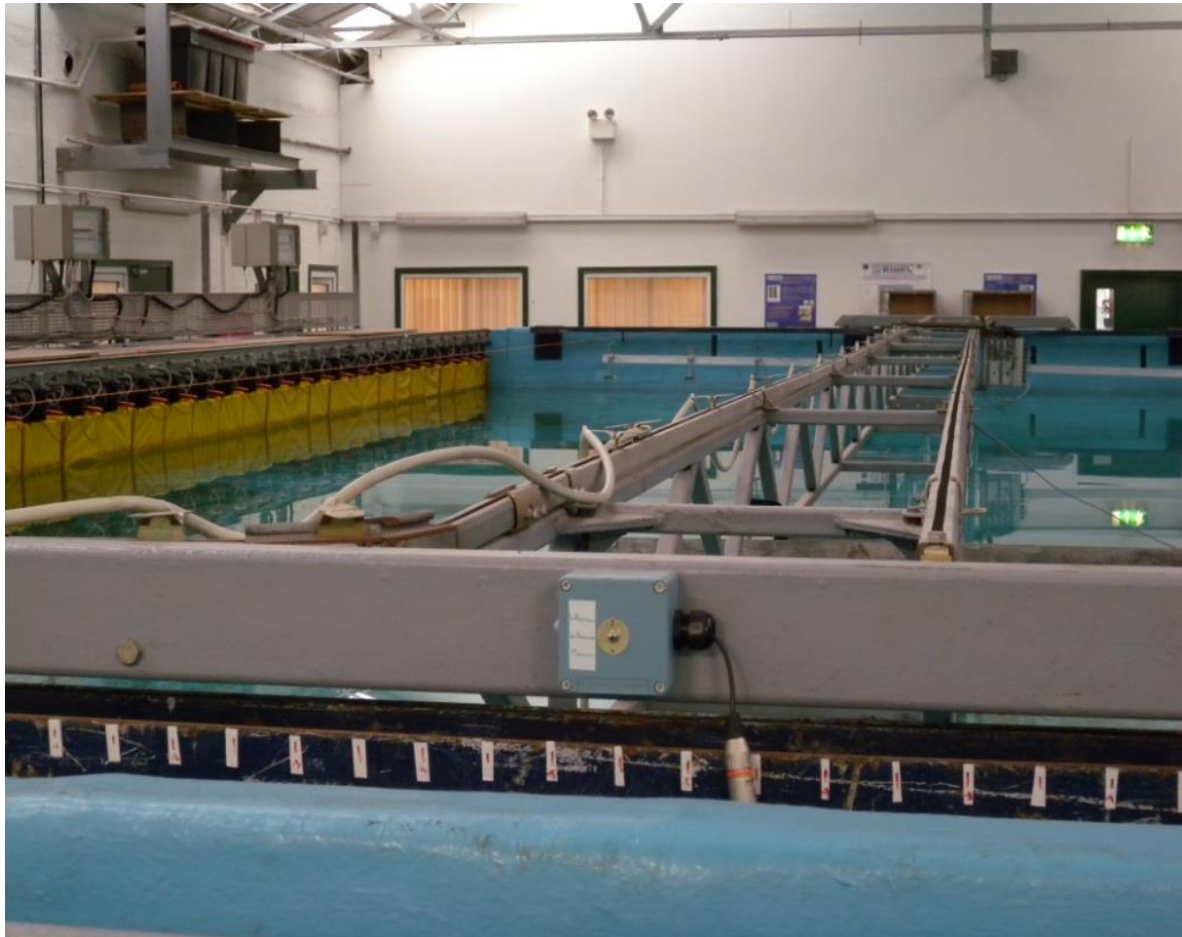
Figure 3:8: Wave Basin with instrument carriage
