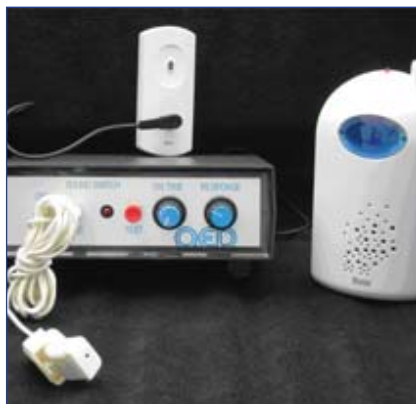
Figure 16 Sound switch with microphone input and alarm output
