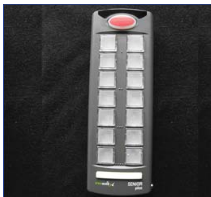
Figure 18 Senior Pilot environmental control unit (for back up use only)
