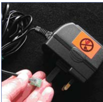
Figure 9 Power cable for infrared telephone
