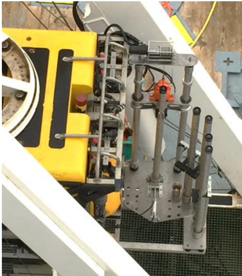
Photograph of Holland 1 ROV with the vibrocoring rig mounted on the front of the vehicle
