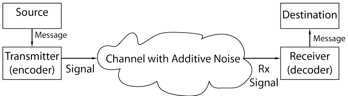
Figure 2.9: Block diagram of a generic communication system
