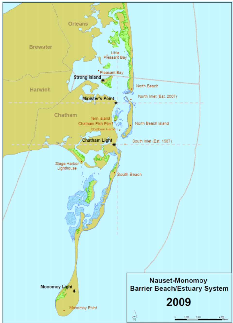
Figure 2.22 Multiple inlet system at the Nauset barrier system, Cape Cod MA. Dominant longshore transport is southerly. Source: Giese et al. (2009).
