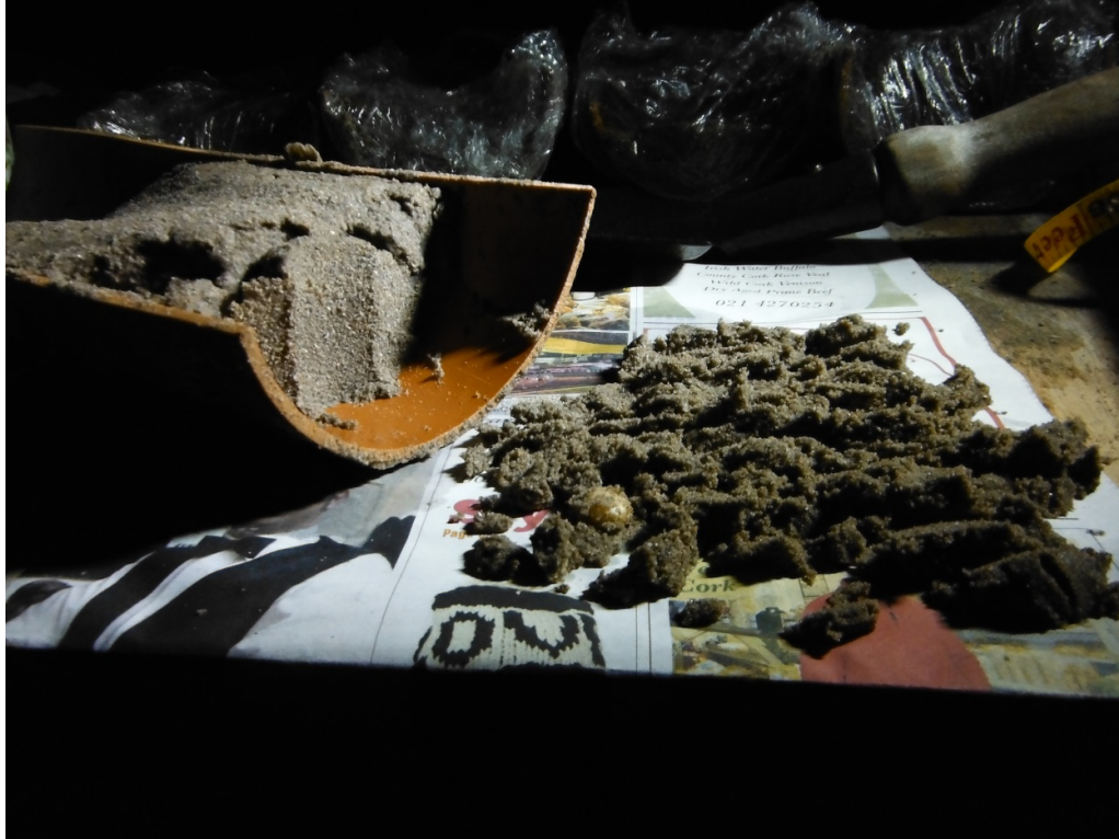
Figure 9.8 Samples from the December tracer experiment were analysed in 1.5 cm layers, whereby each layer was carefully removed, broken, and sifted through. The presence and number of individual tracer particles was noted for each layer.
