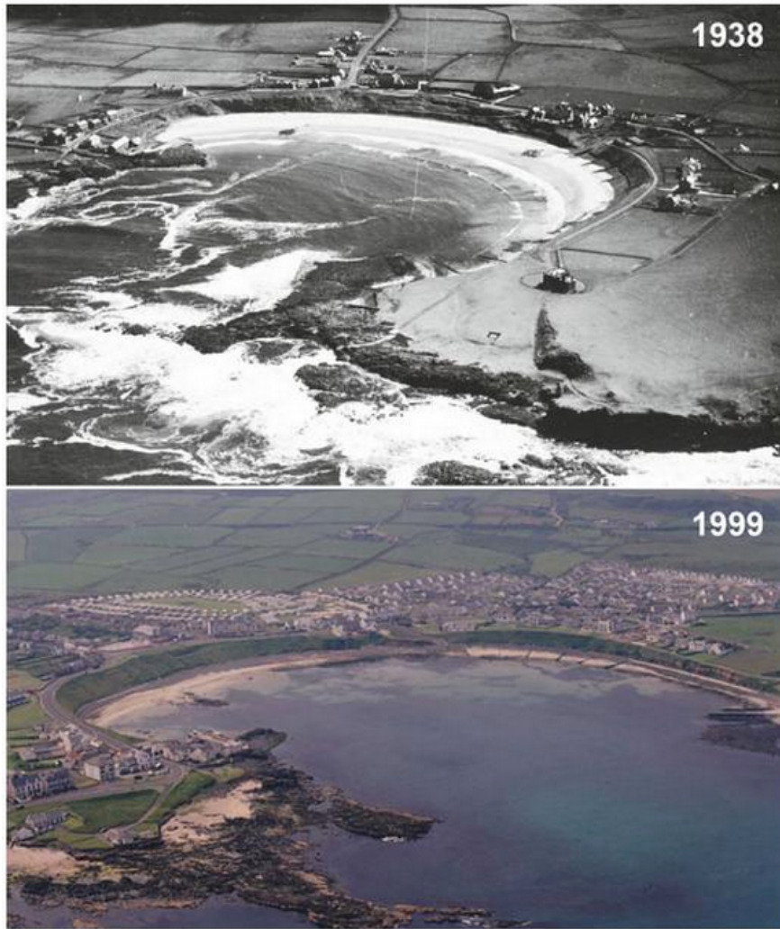
Figure 4.6 Oblique aerial photos of Portballintrae Beach in 1938 (top) and 1999 (bottom) illustrating beach narrowing as a result of the installation of a pier in its western section. Source: Jackson (2012)
