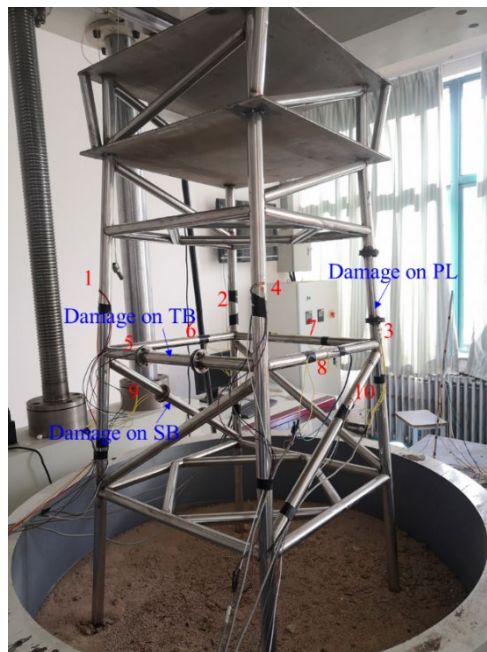
Fig. 16. The placement of the strain gauges and damage locations.
