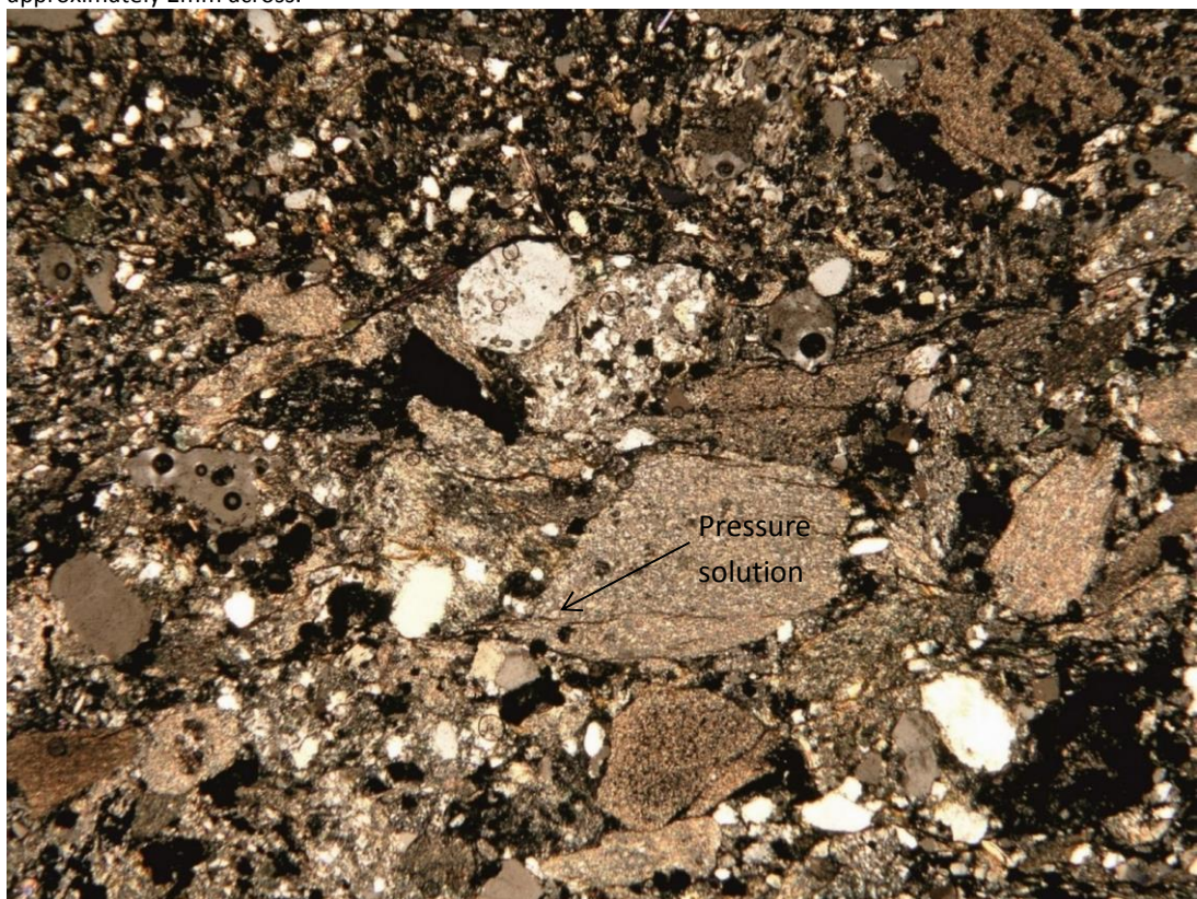
Figure 6. 31 Microstructures observed in a sandy unit from Coumshingaun. A weak pressure solution cleavage is observed, which appears to deform the matrix and lithic clasts equally. Image is approximately 2mm across.
