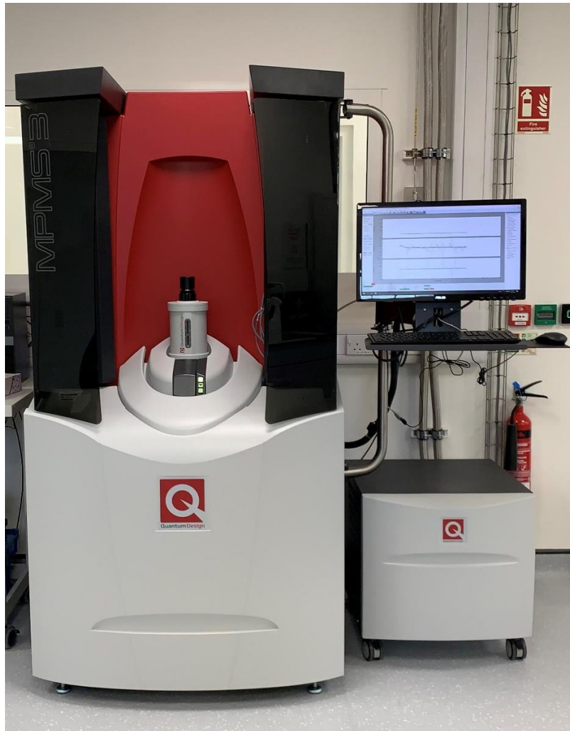
Figure 3.11: Experimental setup of MPMS3 SQUID magnetometer in our laboratory at Tyndall National Institute.
