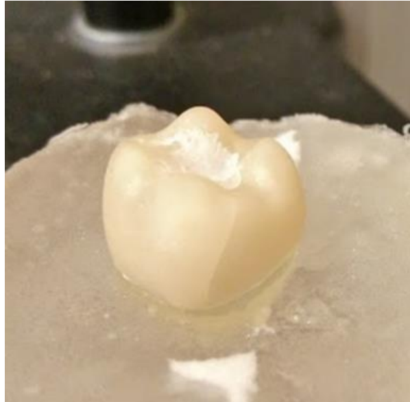
Figure 5.6 An example of a specimen after removal from storage in water at 37°C exhibiting a crack initiated at the distal buccal margin of the LDGC crown and propagated toward the distal cusp on the occlusal surface.
