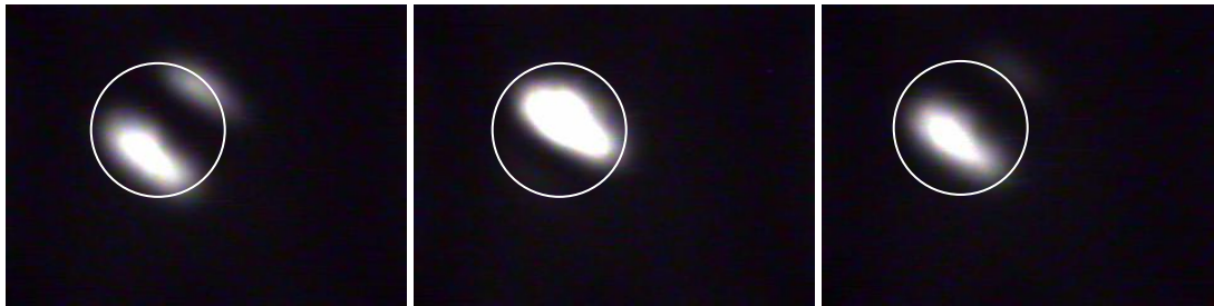
Figure 14: Interferogram of the high soot deposited chip with wavelength tuning.
