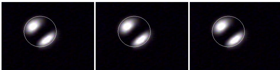
Figure 9: Observed IR interferograms from probe with changes in input polarization.
