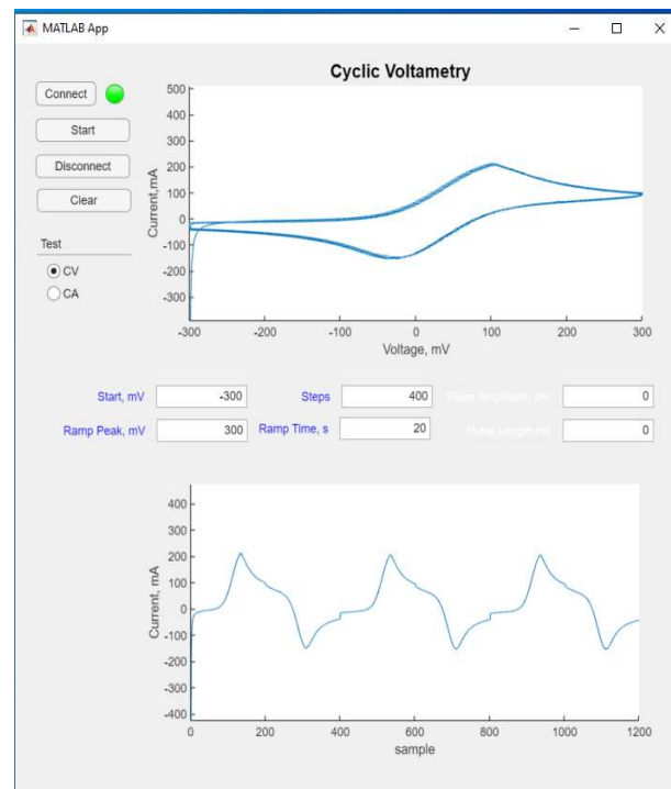
Fig. 6. User interface GUI. Typical CVs of the LIG sensor in aqueous solution containing 5 mM \text{Fe}(\text{CN})_6^{3-} and 0.1M KCl(top). Plot of current versus time (bottom).
