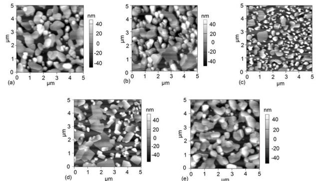
Fig. 6. AFM topography images (a)  $\text{Bi}_5\text{Nb}_0$ , (b)  $\text{Bi}_5\text{Nb}_{0.1}$ , (c)  $\text{Bi}_5\text{Nb}_{0.2}$ , (d)  $\text{Bi}_5\text{Nb}_{0.3}$  and (e)  $\text{Bi}_5\text{Nb}_{0.4}$ .
