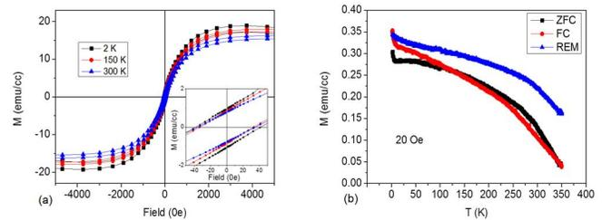
Fig. 10. (a) MH curves after subtraction of the diamagnetic contribution of the substrate magnetic measurements for Bi5Nb0.1. A small magnetic signal of approximately 2.2, 1.6 and 1.5 emu/cm<sup>3</sup> and a  $H_c \sim 40, 36, 34$  Oe at 2, 150 and 300K was detected under zero applied magnetic field (inset (a)). (b) MT graph showing the zero field cooled (ZFC), field cooled (FC) and remnant (REM) curves.
