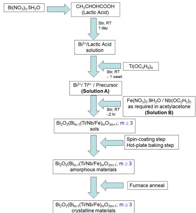
Fig.1. Flow chart depicting the experimental steps involved in preparing the  $\text{Bi}_5\text{Ti}_{3-x}\text{Fe}_x\text{Nb}_x\text{O}_{15}$  ( $m=4$ ) Aurivillius sample series by chemical solution deposition.
