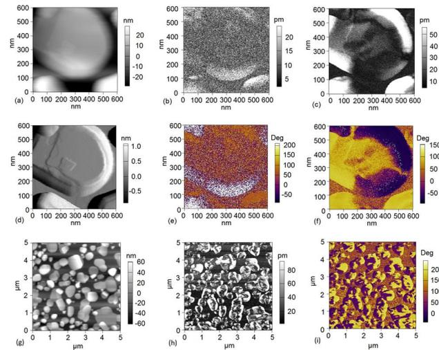
Fig.8. Single frequency PFM measurements of  $\text{Bi}_5\text{Ti}_{2.8}\text{Fe}_{1.1}\text{Nb}_{0.1}\text{O}_{15}$ , (a) height, (b) vertical amplitude, (c) lateral amplitude, (d) vertical deflection, (e) vertical phase and (f) lateral phase. Representative lateral DART PFM images (g) height, (h) amplitude and (i) phase of  $\text{Bi}_5\text{Nb}_{0.1}$  sample.
