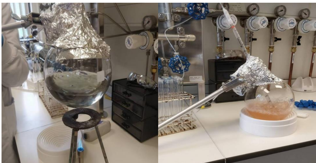
Figure 4.1: Images of boiling and reducing basal medium for methanogen cultivation.
