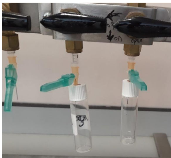
Figure 4.3: Evacuation of stopper-sealed GC vials in preparation for injecting with headspace gas for methane analysis.
