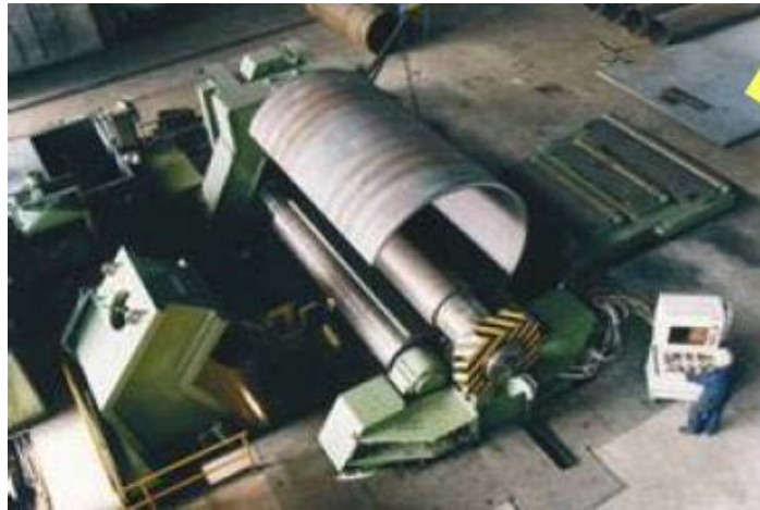
Figure 3-13: Monopile “Can” Rolling
