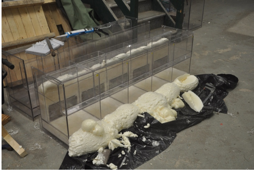
Figure D.5: Expandable foam and ballast blocks in the chamber ballast tanks
