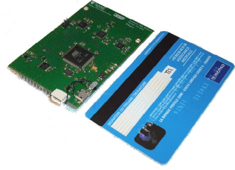
Figure 1. AUTHENTIC Credit Card Form Factor Platform.
