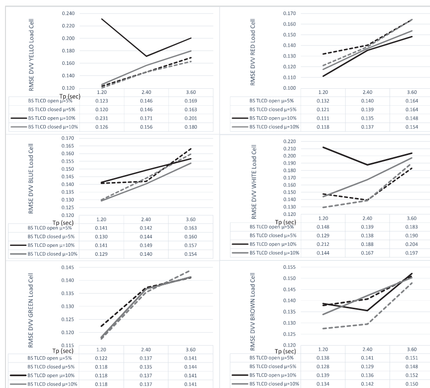
Figure 4: DVV analysis results (RMSE) for Bretschneider spectra waves in function of wave period T_p=1.2, 2.4 , and 3.6 s and frequency f_p=0.83, 0.42 , and 0.28 Hz for TLP with open and closed TLCD ( \mu=5\% and 10\% ).
