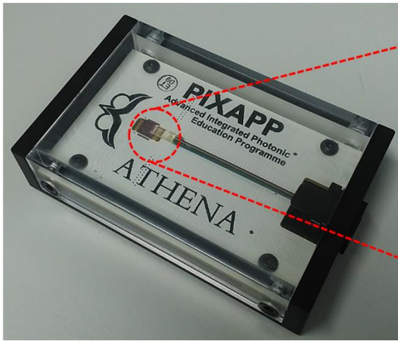
Figure 18: (a) Picture of the PIXAPP Integrated Photonics Educational Kit with the PIC and horizontal fiber array (grating coupled). (b) Closeup image of the PIC and the SOI-Chip.
