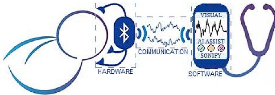
Figure 7.10 Diagram of the App-based variant of the brain stethoscope which consists of portable EEG acquisition, communication and Android app-based interpretation framework. The deep learning algorithms were incorporated into the analytics back-end of the device, which was hosted on a tablet. The Android application was built to visualise the EEG signal and a traffic-light indicator showed the presence of neonatal seizures based on the probabilistic output from a trained model.
