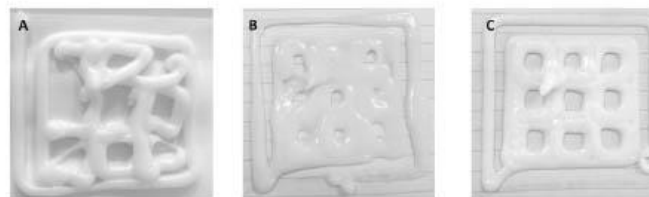
Fig. 7. 3D-printed 40 mm 2 grid: A, Recipe H: Fresh curd control (incomplete grid squares, dragging of mixture causing distorted lines); B, Recipe G: 100% 1–2 month old cheddar (spreading, suboptimal printing precision); C, Recipe D: 25% 1–2 month old cheddar and 75% 6–8 month old cheddar (accurate, clean lines, very little spreading, optimal printing precision).
