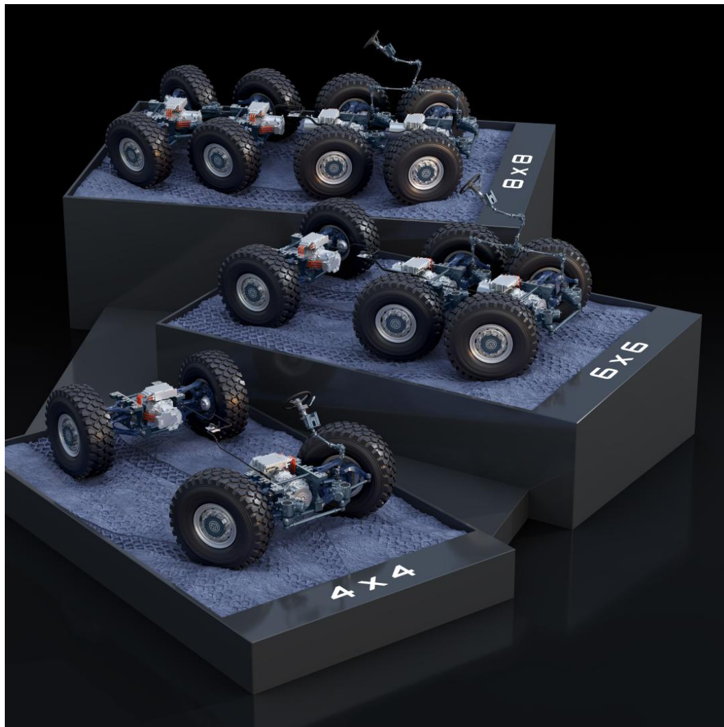
Fig. 1.5: A CAD rendering of 4x4, 6x6 and 8x8 drivelines.
