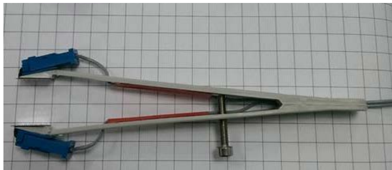
Figure 2. Completed device showing electrical connections and stopper screw.
