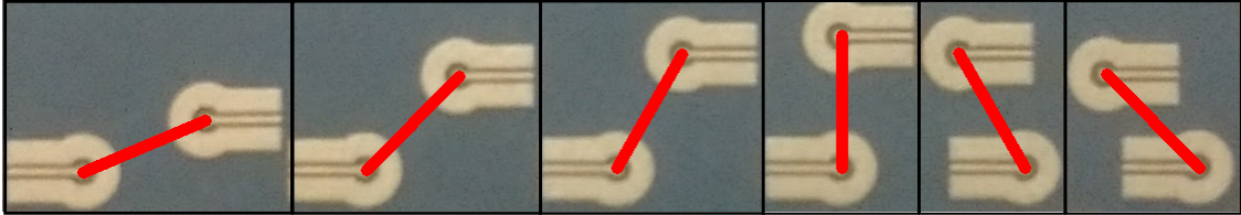
Figure 2: The transition allows rotation at an arbitrary angle
