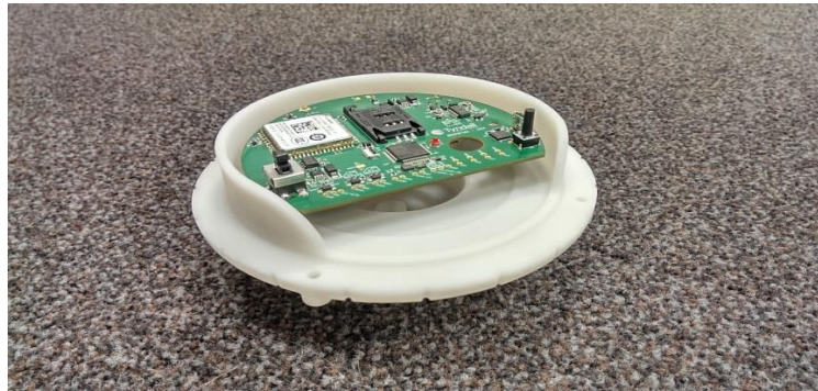
Figure 5. System Enclosure, lower half with PCB placed
