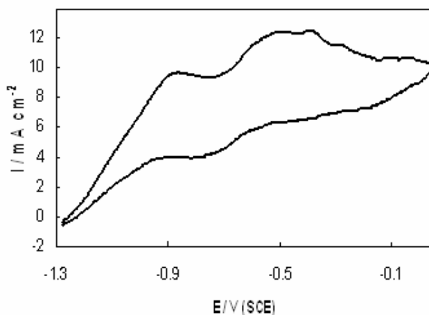
Figure 14. Cyclic voltammogram for segmented NPG-Au wire array on a planar Au film in 1.0 \text{ mol dm}^{-3} NaOH containing 0.02 \text{ mol dm}^{-3} AB at 10 \text{ mV s}^{-1} .
