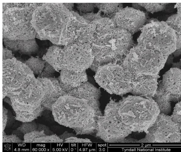
Figure 7. SEM image of NPG-coated Au wire array on Au.
