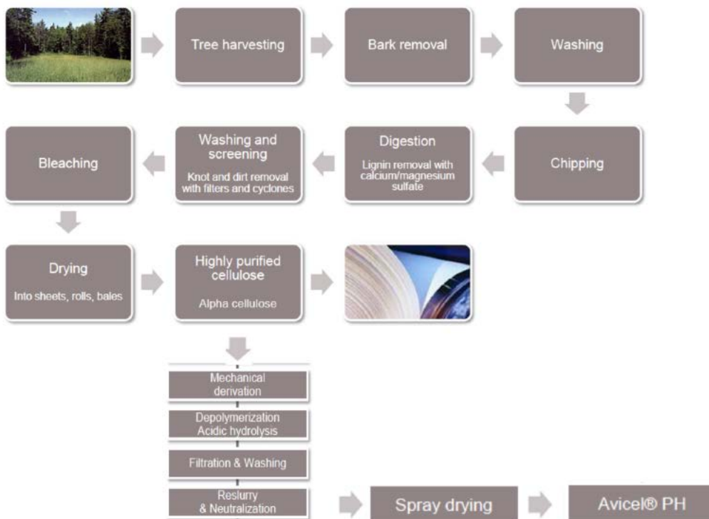
Figure 4. Schematic overview of MCC production process (Avicel® PH). Reproduced with permission from DuPont Nutrition and Health.
