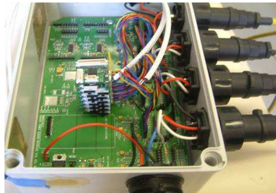
Figure 2: Multi-sensor interface board with sensors
