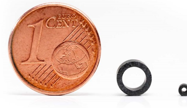
Figure 22. T6 and T2 cores to test complex permeability characteristic.
