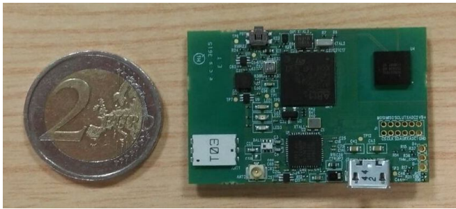
Fig. 1. Tyndall Wireless Inertial Measurement Unit (WIMU).
