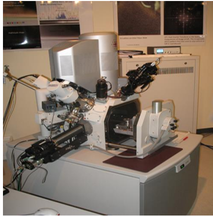
Figure 2.6: An example of an FEI Quanta 3D Dual Beam FIB. Reference [20].
