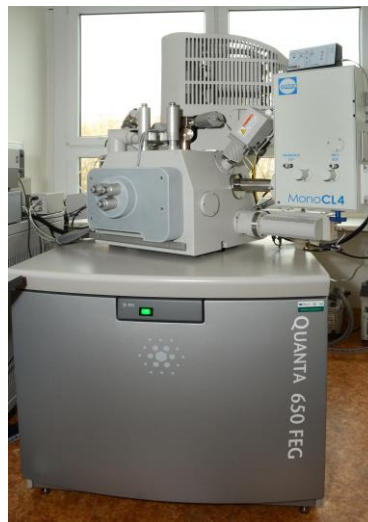
Figure 2.5: An example of an FEI Quanta 650 FEG SEM. Reference [12].
