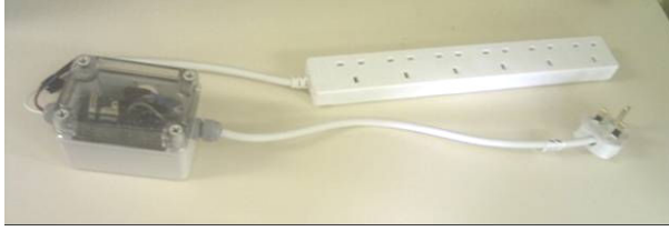
Figure 2. REAM node in enclosure with attached extension board and plug
