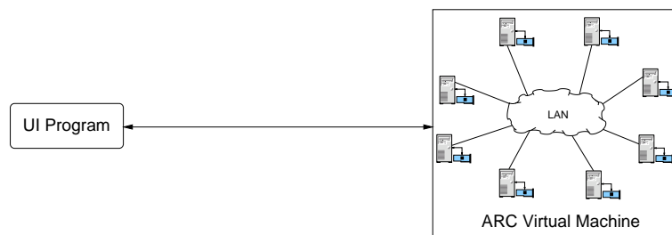
Figure 2.2: At runtime, users start, stop and monitor application instances via the UI program. ARC daemon instances and computation processes executing on each cluster node create the illusion of a single virtual machine.
