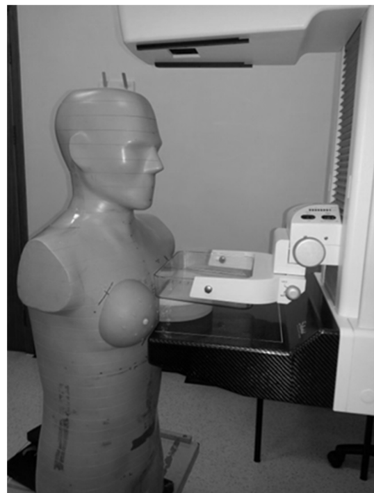
Figure 1. ATOM and breast phantoms positioned on a FFDM machine in the cranio-caudal (CC) position.
