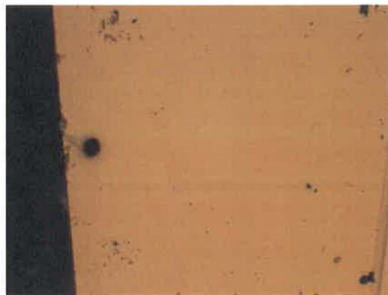
Figure 2: An example of the platinum deposition achieved on a copper coated substrate.
