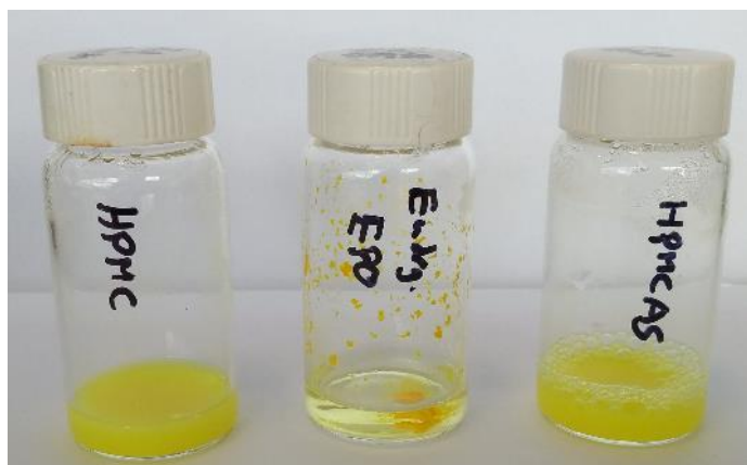
Figure S 4. PI test samples of sLBF-PI with HPMC, Eudragit ® EPO and HPMCAS after 180 min in FaSSIF. Agglomeration of Eudragit ® EPO can be observed.
