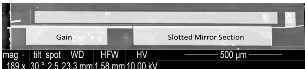
Fig 2.7: Single facet SFP laser with angled output on the right side to minimise reflections from the facet.
