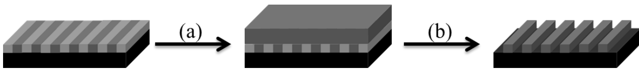
Scheme 2: Schematic diagram of the fabrication of Iron oxide nanowires: (a) spin-coating of 0.4 wt% of Iron (III) nitrate nonahydrate ( \text{Fe}(\text{NO}_3)_3 \cdot 9\text{H}_2\text{O} ) in ethanol, (b) UV/Ozone treatment to generate iron oxide nanowires on Silicon substrate
