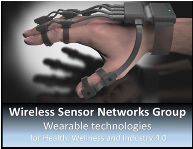
Fig. 1. Tyndall HCI glove-like system
