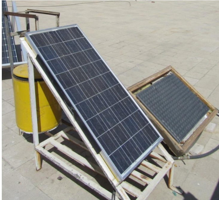
Fig. 3. PV/T collector system
