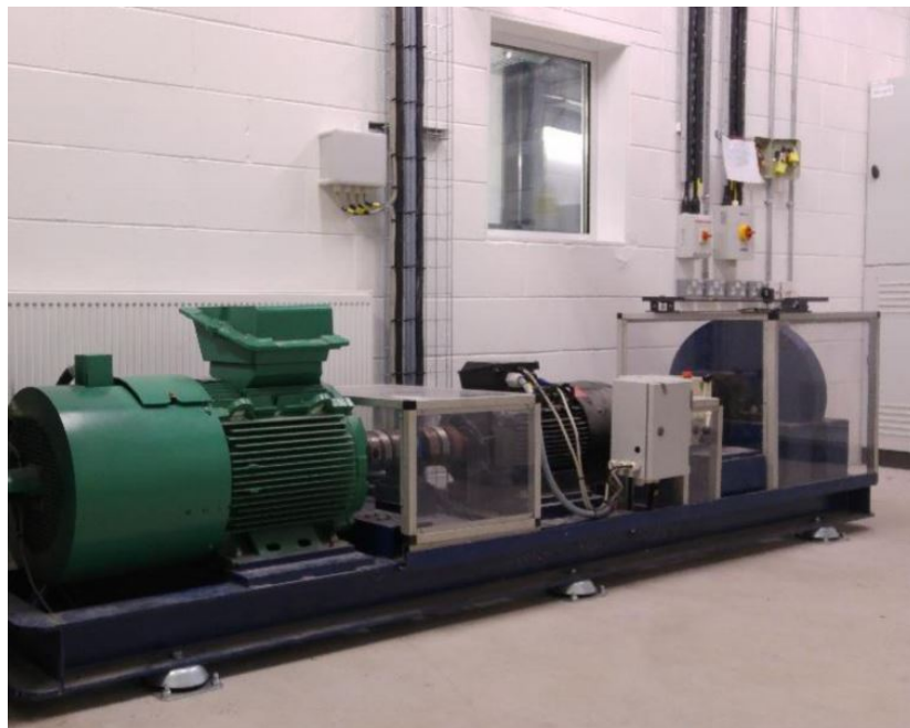
Figure 13. Rotary test rig of the Lir National Ocean Test Facilities (Lir-NOTF), used to emulate the turbine-generator systems of the devices.
