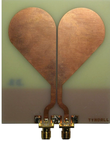
FIGURE 3: Photograph of the physical implementation of the folded planar differential antenna ( \rho = 45^\circ , D = 3 cm).
