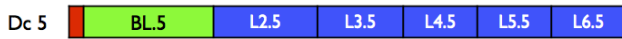
Fig. 5 SD packetisation of D_c 5 from ALD in Figure 2. It can be seen that each packet contains section segments from all layers (red denotes packet header)
