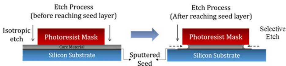
Fig. 1. (a) Isotropic etch process before reaching seed layer. (b) Selective etch behaviour after reaching seed layer.
