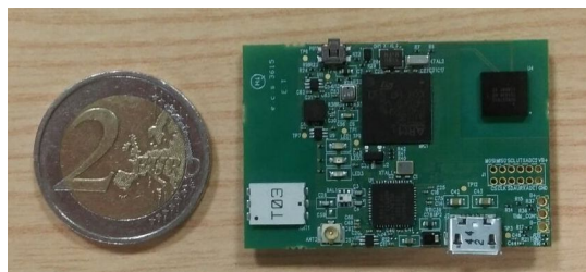
Figure 1. Tyndall Wireless Inertial Measurement Unit (WIMU).
