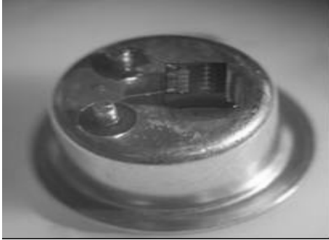
Figure 2. Schematic view of the pressure sensor
