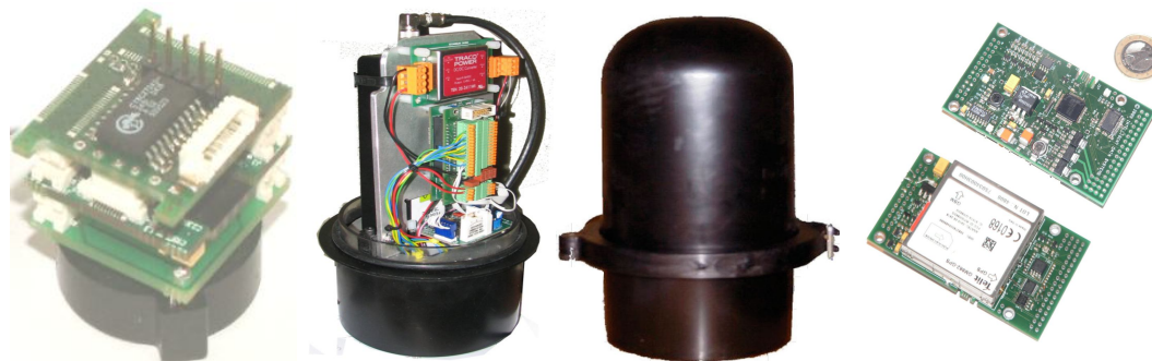
Figure 2. PSOC reconfigurable sensor interface on the Tyndall Stack and IDS DataPOD electronics
