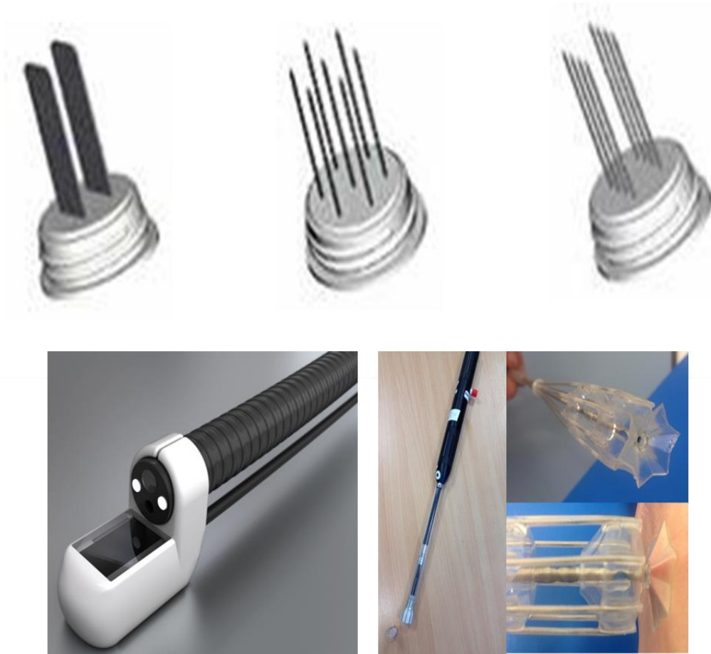
Figure 1.3: (Top: L – R) Plate electrodes; hexagonal array needle electrodes; parallel array needle electrodes. (Bottom: L – R) EndoVe, a novel electrode system designed for delivery of electroporating pulses to gastrointestinal tissues and tumours; ThoraVe, a novel electrode device designed for delivery of electroporating pulses to pulmonary tissues and tumours. The choice of electrode used for electroporating is influenced by a number of factors, including tumour locale, the pliability of the tissue to be electroporated, the likelihood of encountering resistance (e.g. previously irradiated skin) and physician preference.
